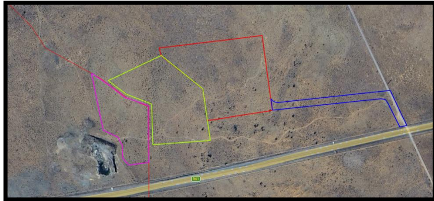
Figure 6: Alternative layout option (Alternative 2) Quarry area (yellow polygon), laydown area (red polygon) with the viable access road (blue line) within the surrounding landscape.
