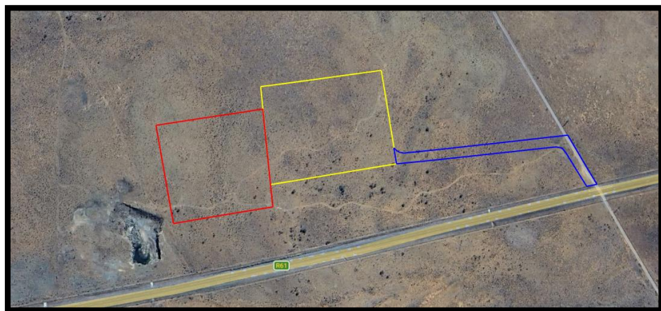
Figure 5: Satellite view showing the position of Site Alternative 1 Quarry area (red polygon), laydown area (yellow polygon) with the viable access road (blue line) within the surrounding landscape.
